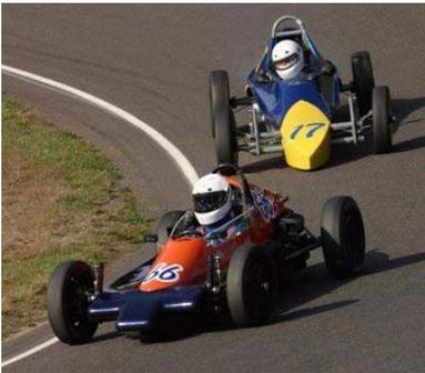
Formula Vee is a very long running spec. series based on older Volkswagen components including engine, transmission, front suspension, brakes, and wheels. Newer cars are better aerodynamically but older cars are still competitive making this a great budget class.
