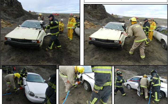
ABOVE: Door Removal 101: Pinch the fender to open a gap at the door fender interface. Peel back the door to access and break the hinge. Force the door back and attack the striker pin. This technique is bound to leave a mark.
