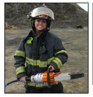
The Hot Rod of the emergency tool world! Single hose non-kink hydraulics, twist grip control, aluminum and titanium construction, quiet running hydraulic pump and power to lift a Freightliner. This tool represents the latest successor generation to the Hurst Jaws of Life.
