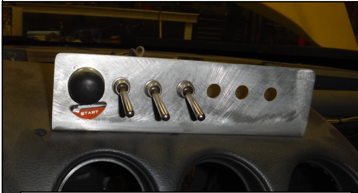
Switch panel, off is down. Make shutting off all switches part of your emergency exit practice.
